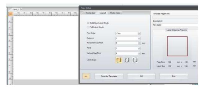
When the number of horizontal columns and the number of vertical lines is 2, the preview of the label design area is as follows:
